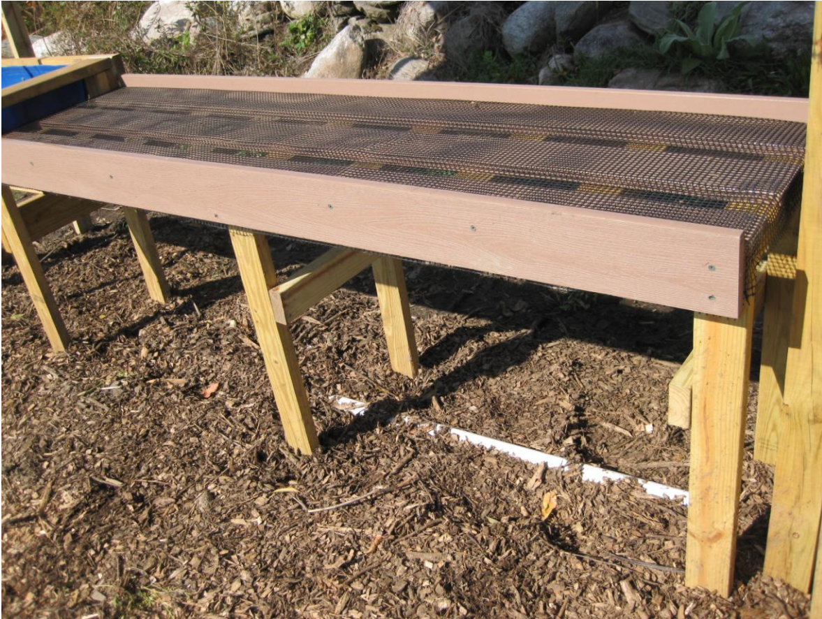
Figure 5. Large drying rack with plastic lumber and PVC mesh top
