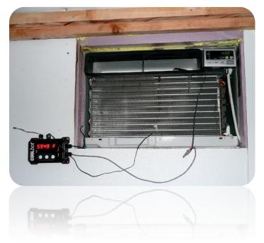
the front panel to access the fins) in order to detect the formation of frost, at which point it forces the A/C to run a defrost cycle. The top wire on the side is a power cord, and the bottom wire on the side is a small electrical heater which you wrap together with the A/C temperature sensor, using a small piece of aluminum foil, to trick it into thinking that it needs to be running. Notice that the top panel has been removed as well, since it limits airflow.
